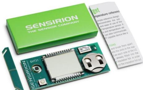
The SHT31 Smart Gadget is a reference design circuit board which demonstrates the outstanding performance and ease of use of Sensirion's humidity and temperature sensors. It not only shows humidity and temperature values on the display, but it can also communicate wirelessly with a Bluetooth Smart enabled device like a smartphone. It comes with a battery.
